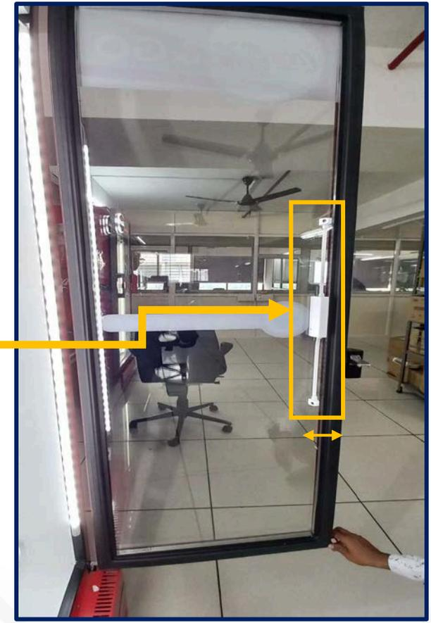
Ensure that the device is installed the same as shown in the below image (Barcode should be facing toward the magnet).
