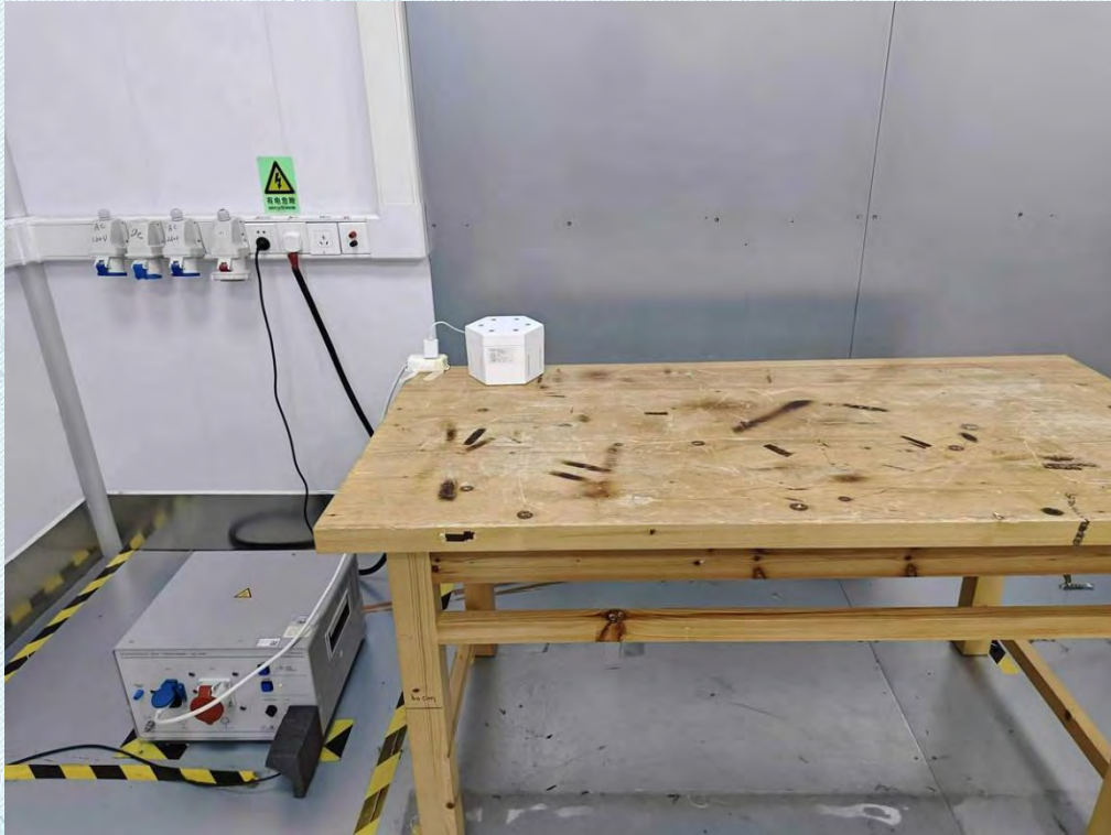
Conducted Emission at AC power line
