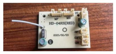
Remarks: The specification of 2.4G antenna is 17-core bare copper wire with an outer diameter of 1.6MM, white, with a length of 35MM, and the end of the wire is stripped 3MM and tinned. Meet the environmental protection standards: EU EN71(19E), ROHS, PAHS, 6P~16P, Europe and America CPSIA, HR4040.
