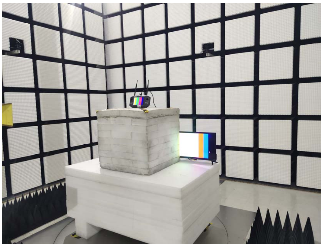
Radiated Emission Above 1GHz View
