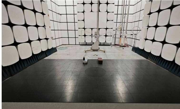
Radiated emission 30MHz~1GHz
