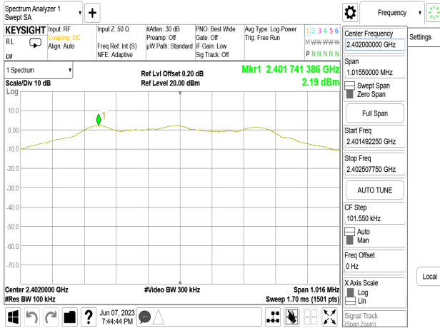
Reference Level_BLE 1M_MidCH20-2442MHz
