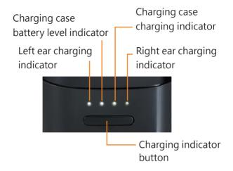
Press the charging indicator button to observe the charging status of the hearing aid and charging case.
