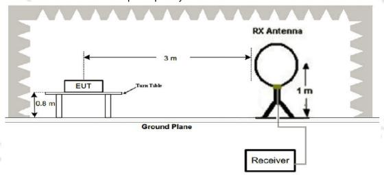
2. Radiated Emission Test-Up Frequency 30MHz~1GHz
