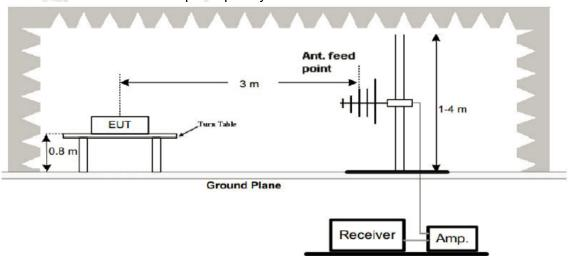
3. Radiated Emission Test-Up Frequency Above 1GHz
