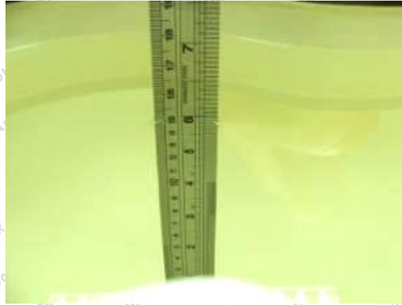
Photo of Liquid Height for Head SAR
