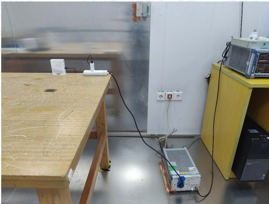
Photo of Setup for Conducted Emission
