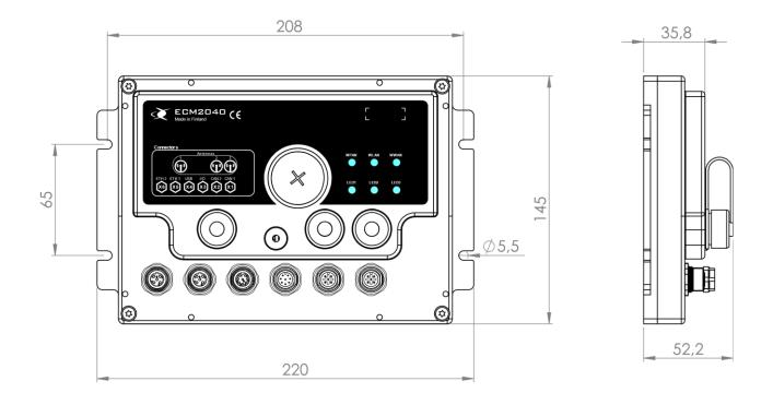
The preferred mounting position is connectors pointing downwards. If the unit is mounted connectors pointing to the side, then it is vital to leave some loose cable with a downward cue to prevent the ingress of moisture through connector.
