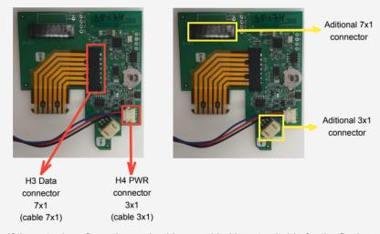
If the actual configuration and cables provided is not suitable for the final product additional 7x1 and 3x1 connectors are available.
