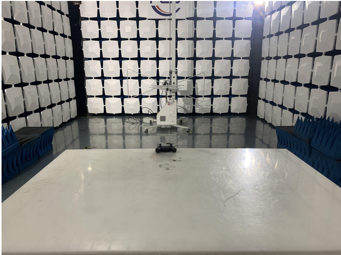
Above 1GHz for radiated emission test setup
