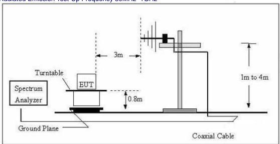
(C) Radiated Emission Test-Up Frequency Above 1GHz
