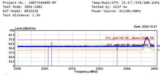
Trace: 1 Freq Reading Factor Result Limit Margin Polarity Remark MHz dBuV dB/m dBuV/m dBuV/m dB 2362.27 30.57 45.65 54.00 vertical 15.08 8.35 Average 2363.69 27.96 30.59 58.55 74.00 15.45 vertical Peak Average 2390.00 14.35 30.93 45.28 54.00 8.72 vertical 2390.00 24.64 30.93 55.57 74.00 18.43 vertical Peak
