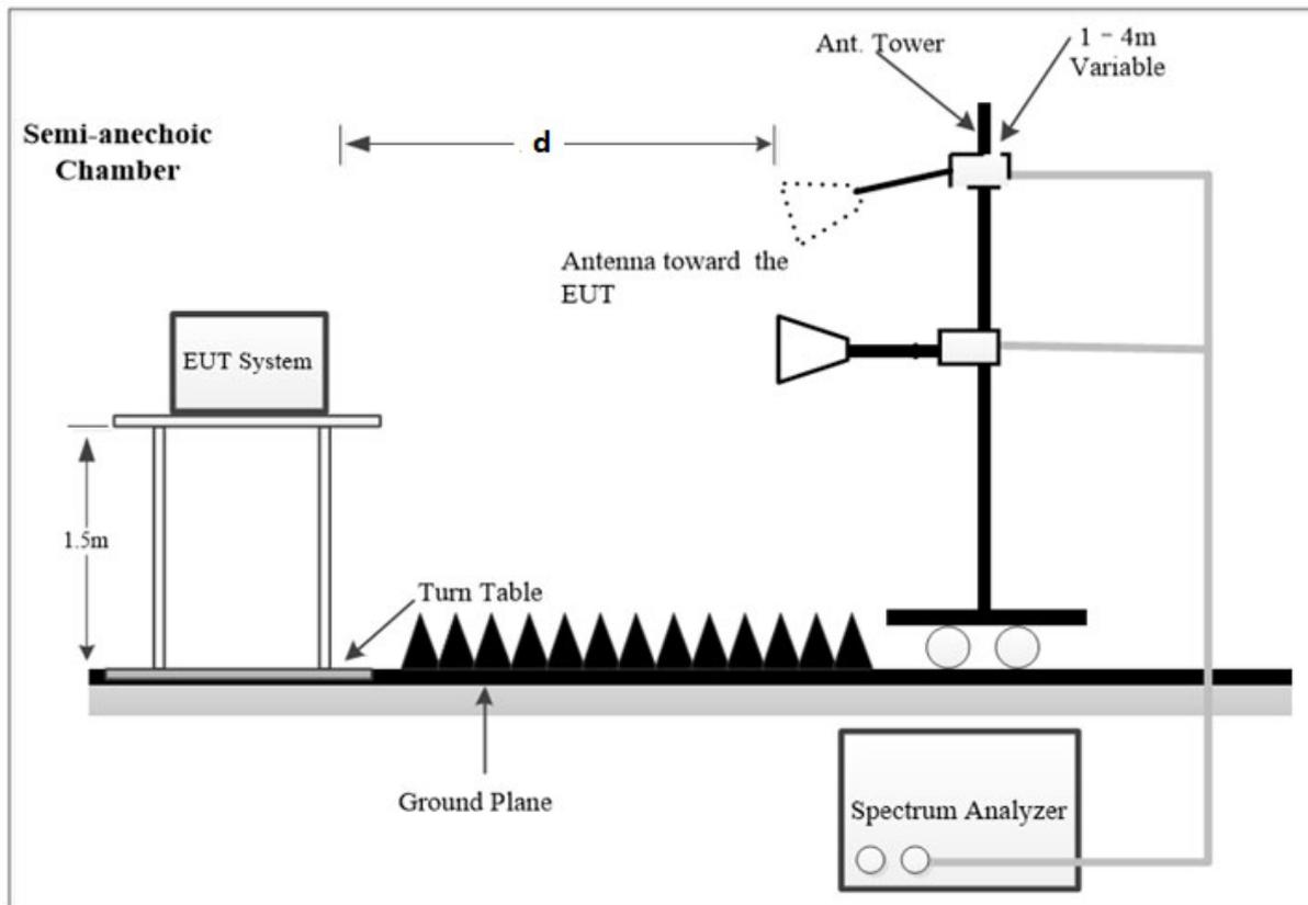
The radiated emission tests using the setup accordance with the ANSI C63.10-2020. The specification used was the FCC 15.209 and FCC 15.247 limits.
