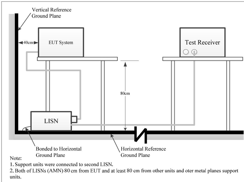
The measurement procedure of EUT setup is according with ANSI C63.10-2020. The related limit was specified in FCC Part 15.207.
