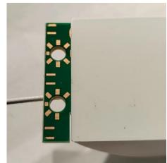
3. The antenna must be installed in place and secured with plastic parts
