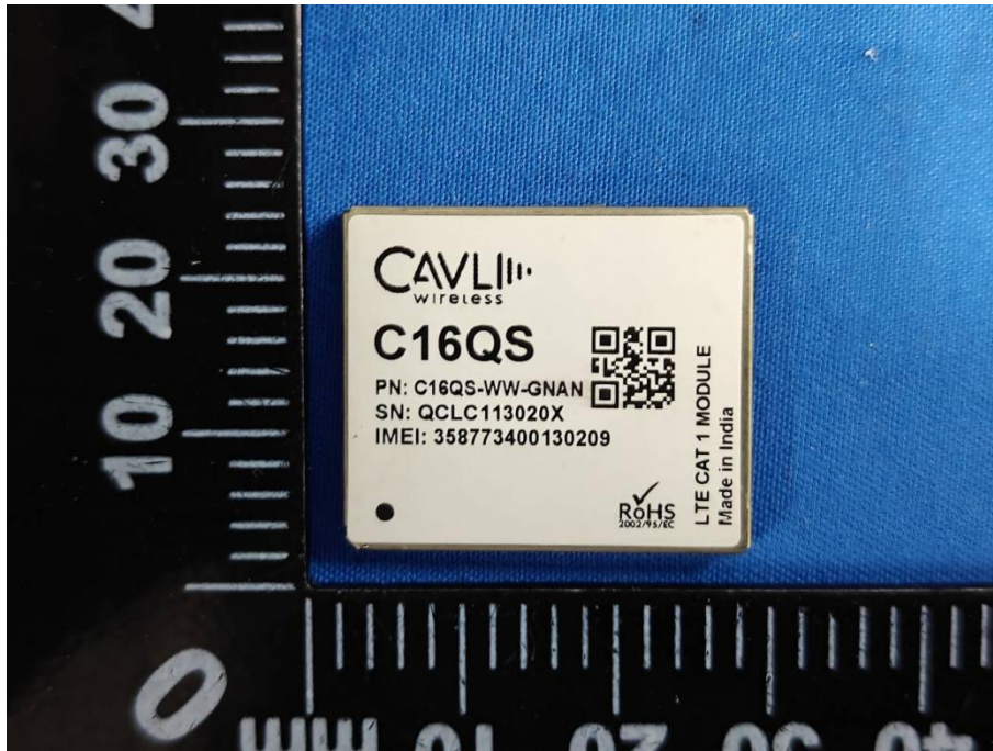
EUT TOP VIEW (WITH SHIELDING)
