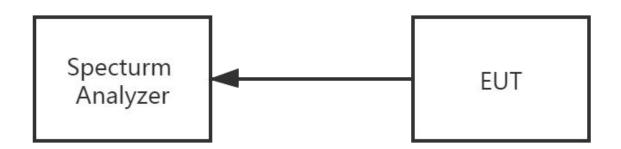
The EUT which is powered by the \${ Power }, is connected to the Spectrum Analyzer; the RF load attached to the EUT antenna terminal is 500hm; the path loss as the factor is calibrated to correct the reading.
