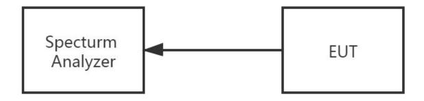
The EUT which is powered by the \${ Power }, is connected to the Spectrum Analyzer; the RF load attached to the EUT antenna terminal is 50Ohm; the path loss as the factor is calibrated to correct the reading.
