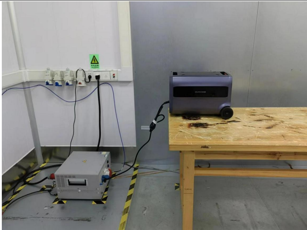
Conducted Emission at AC power line
