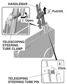
Close the telescoping steering tube clamp. Close the lower clamp.
