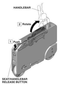
Open the telescoping steering tube clamp. Pull and lift the handlebar. Make sure you hear a click when the tube locks into place.
