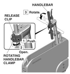
5. Close the rotating handlebar clamp. Make sure you hear a click and the handlebar is clamped tightly.
