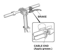
2. Apply grease to the brake cable location shown.
