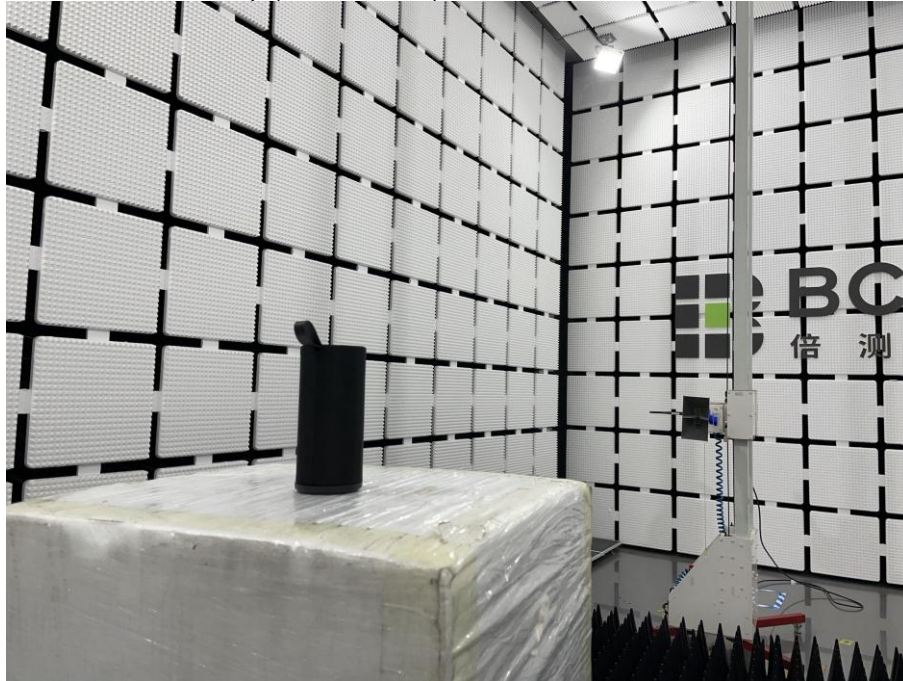
Spurious Emission Test Setup (Above 1GHz)
