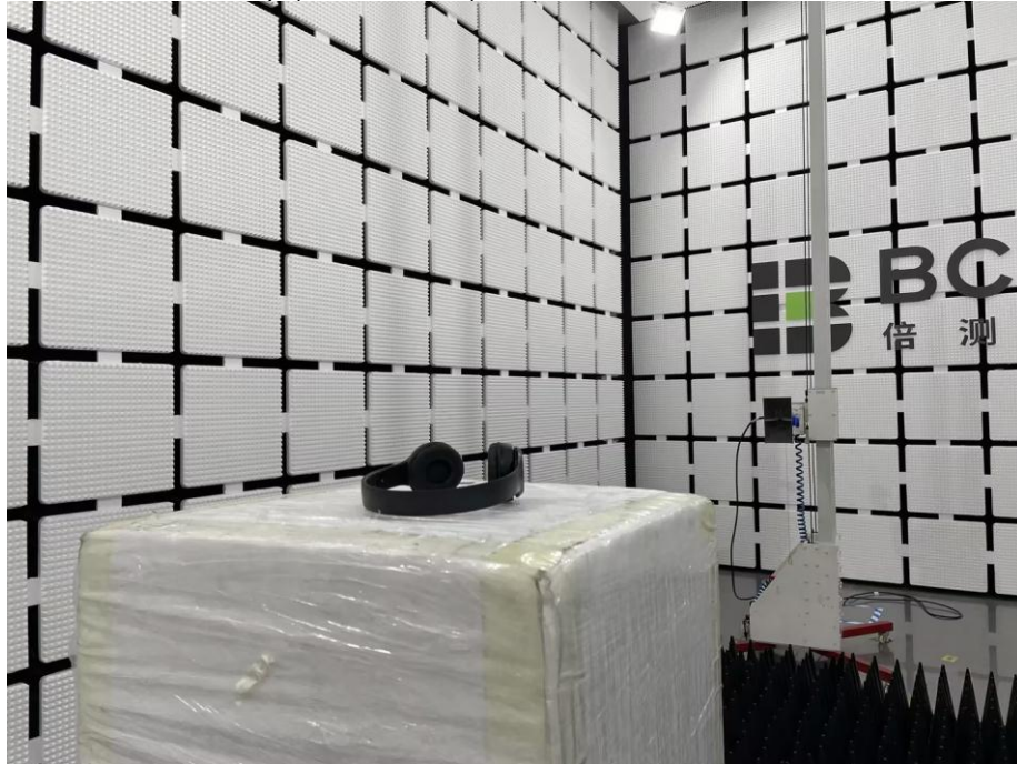
Spurious Emission Test Setup (Above 1GHz)
