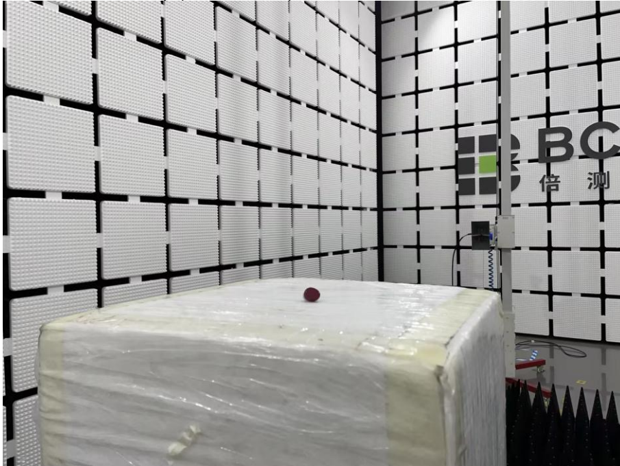
Spurious Emission Test Setup (Above 1GHz)
