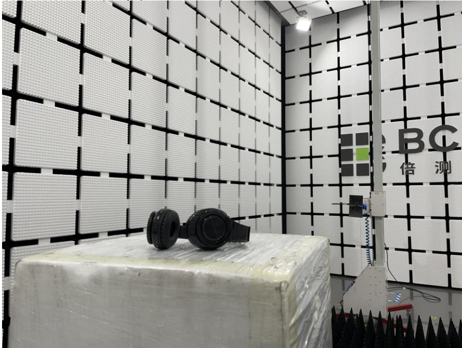
Spurious Emission Test Setup (Above 1GHz)
