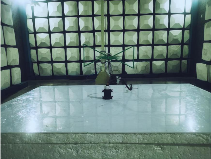
RF Radiated Test (1-18GHz)
