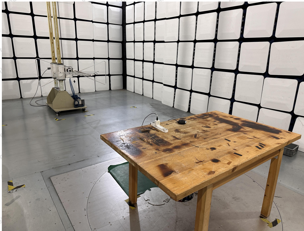
Photo of Radiation Emission Test
