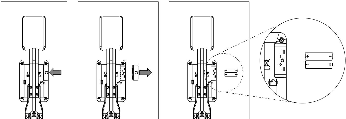
A weak or an extinguished computer display makes a battery change necessary. The computer is equipped with four batteries. Perform the battery change as described below:
