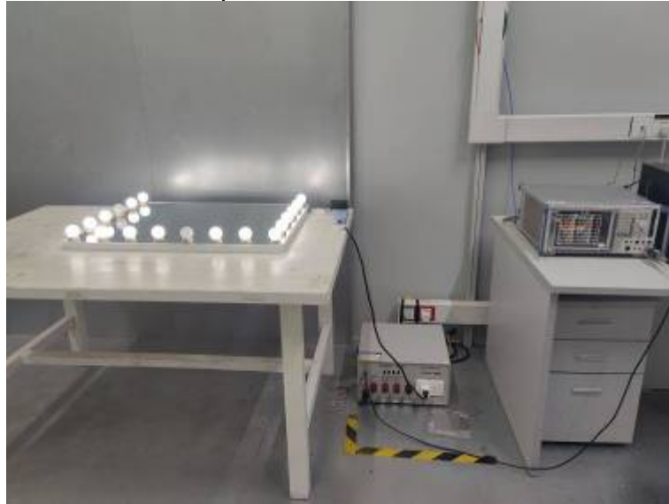
Photos of power line conducted emission test
