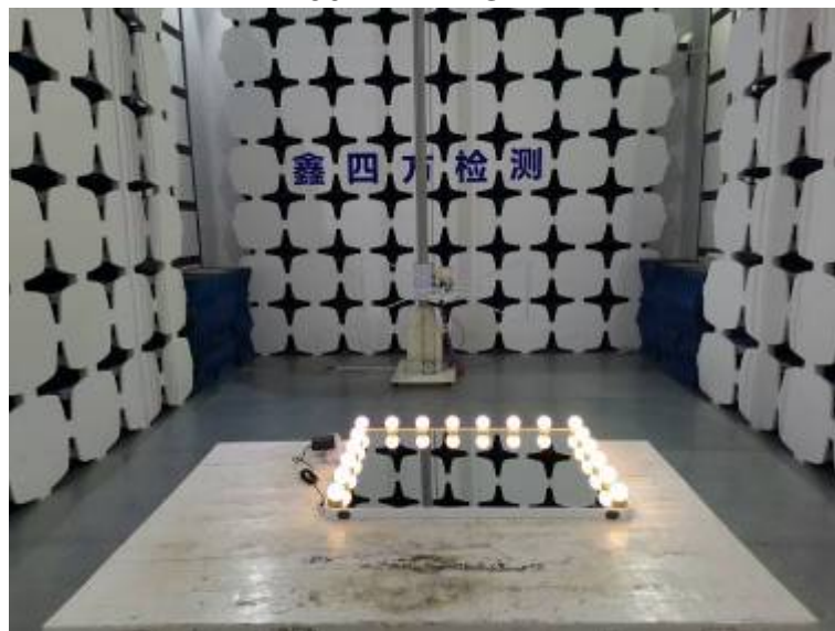
Photos of radiated emission test 30MHz – 1GHz
