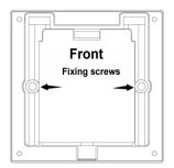
(c) Read the head panel and read the head body snap together, first from the upper snap down and then press the lower and bottom screw hole alignment; finally in the bottom of the anti-theft screw hole screwed on the countersunk head machine wire within the plum security screws fixed, as shown in the figure below.
