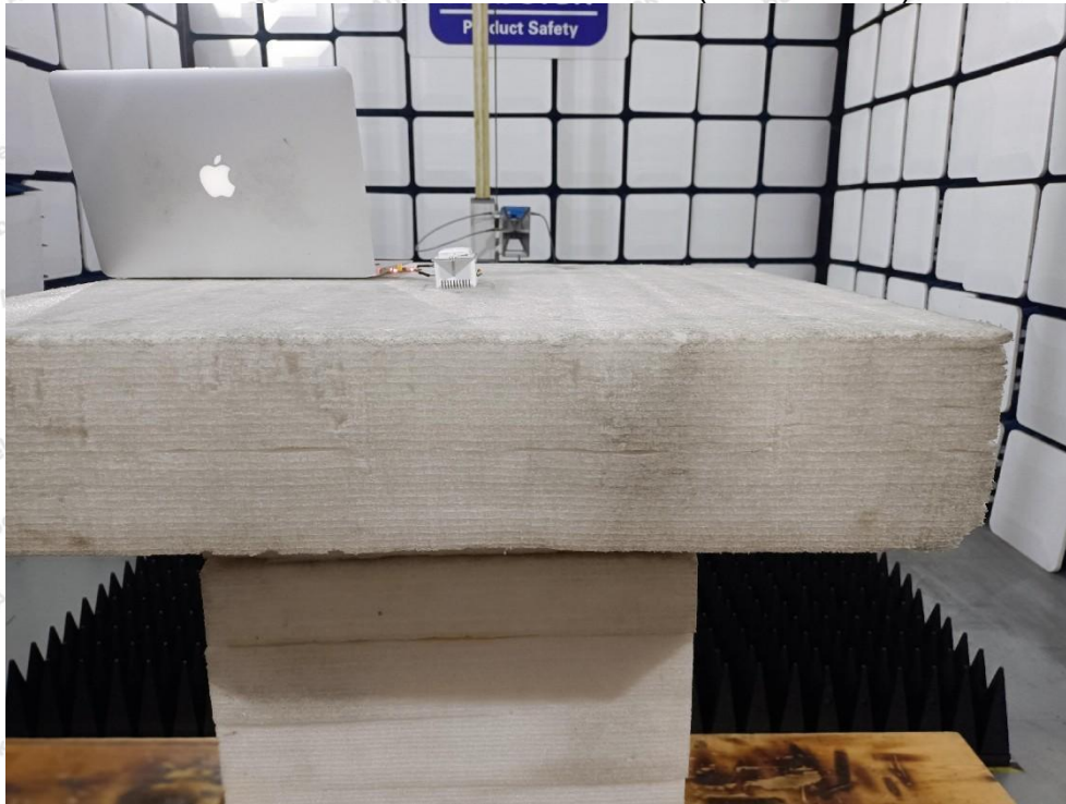
Photo of Radiation Emission Test (above 1GHz)
