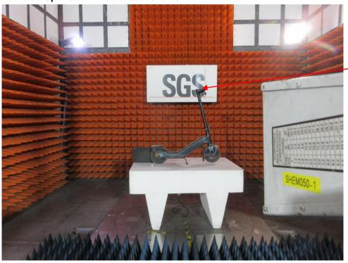
RF antenna and module are located in the handle at above 1.5m from the floor.
