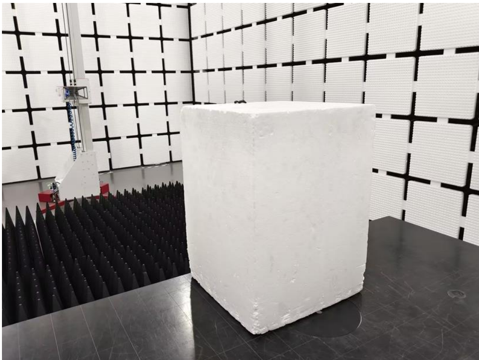
Spurious Radiation Emissions Test (>1G)
