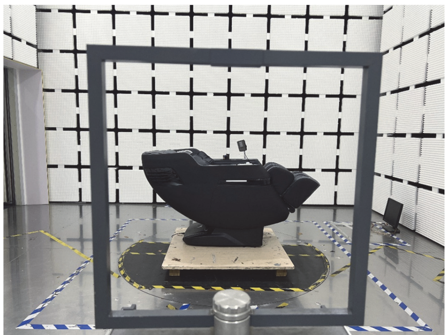
Radiation Emission Test Setup (Below 30MHz)
