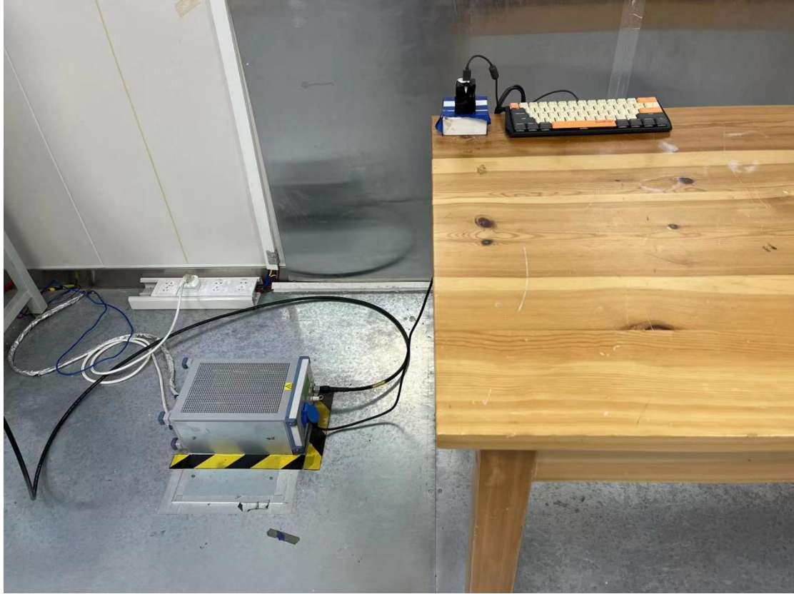
Conducted emission test setup
