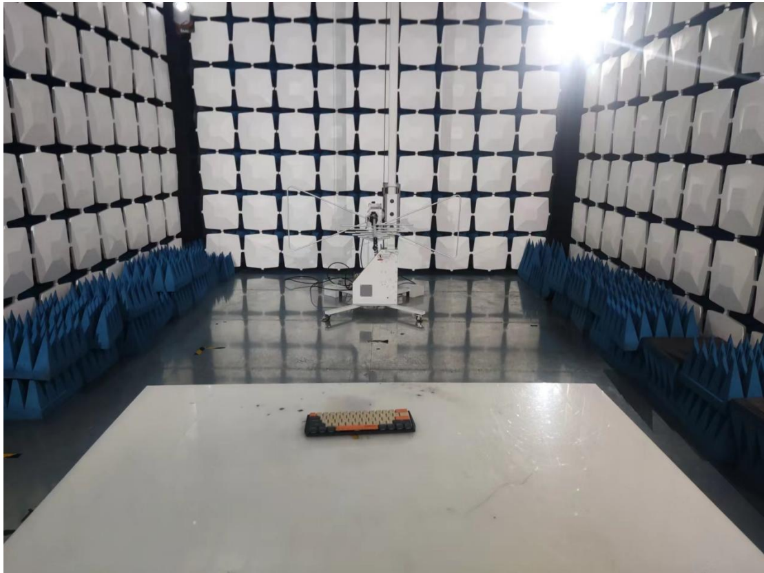
Blow 1GHz for radiated emission test setup
