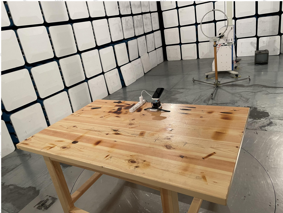
Photo of Radiation Emission Test
