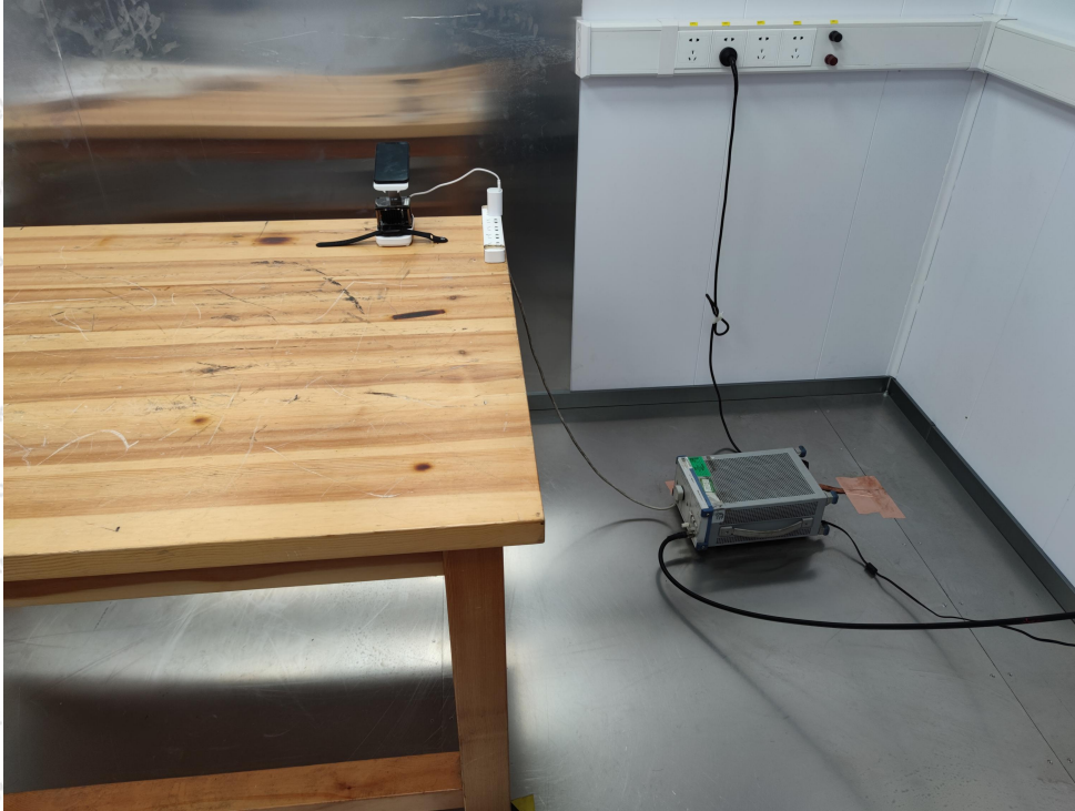
Photo of Conducted Emission Measurement
