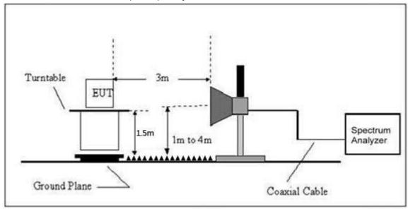
Frequency:9kHz-30MHz RBW=10KHz, VBW =30KHz Sweep time= Auto
