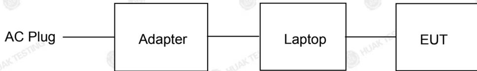
Operation of EUT during above 1GHz Radiation testing:
