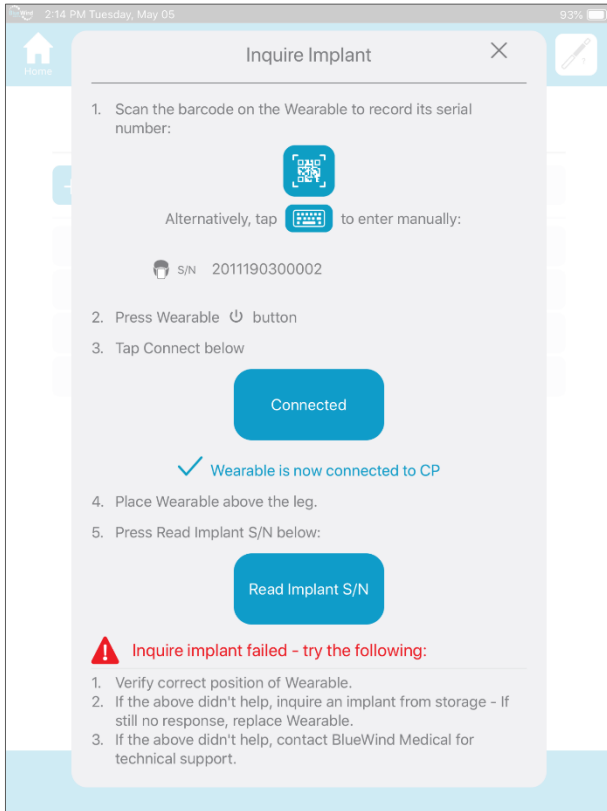
Figure 33 Inquire Implant failed
