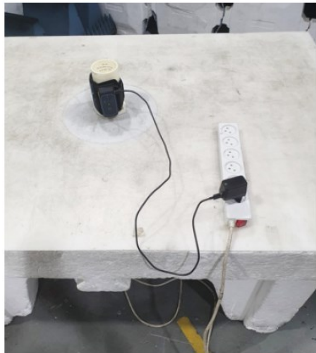
Picture # 7. Radiated emission test setup – Charging mode
