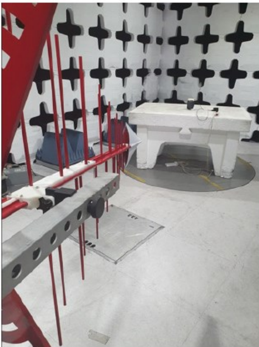
Picture # 7. Radiated emission test setup – Charging mode
