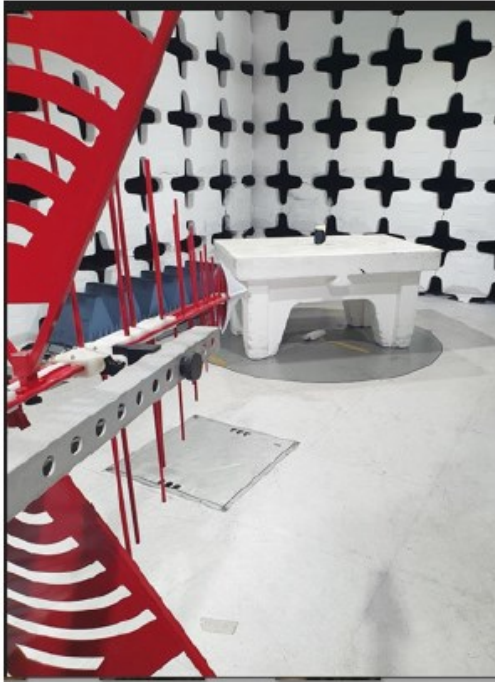
Picture # 6. Radiated emission test setup - Operation mode
