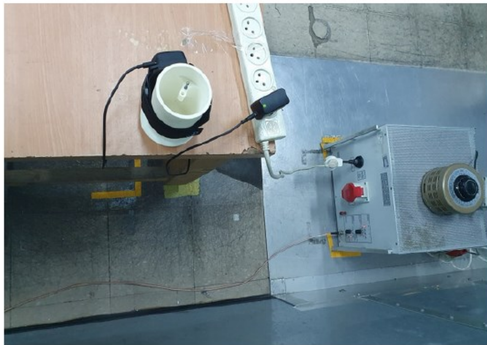
Picture # 9. Conducted emission test setup with Power Adapter 1
