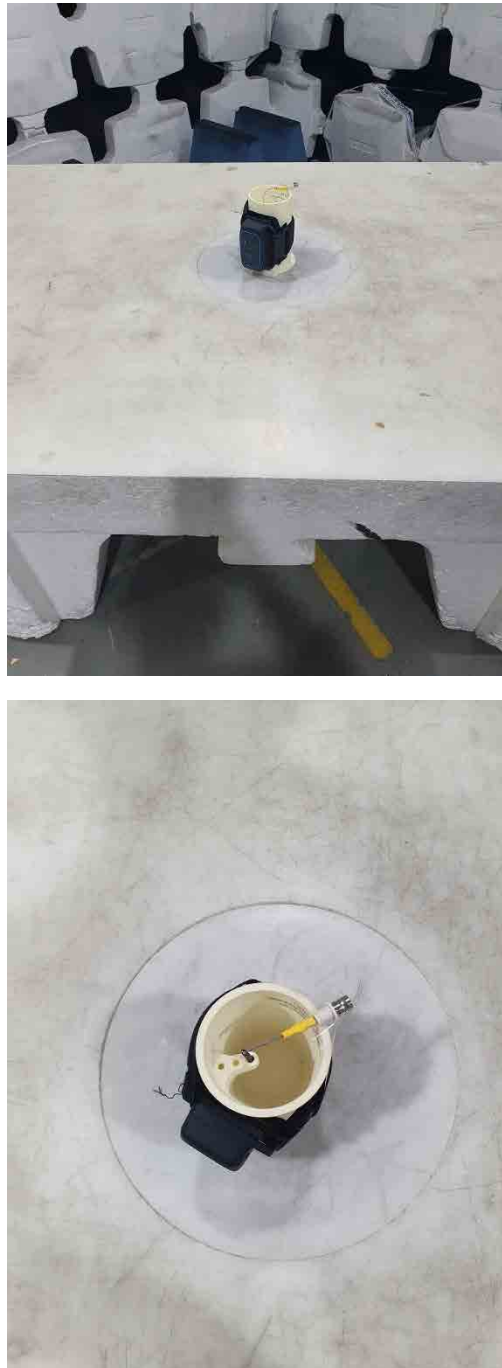
Picture # 7. Radiated Emission test setup.
