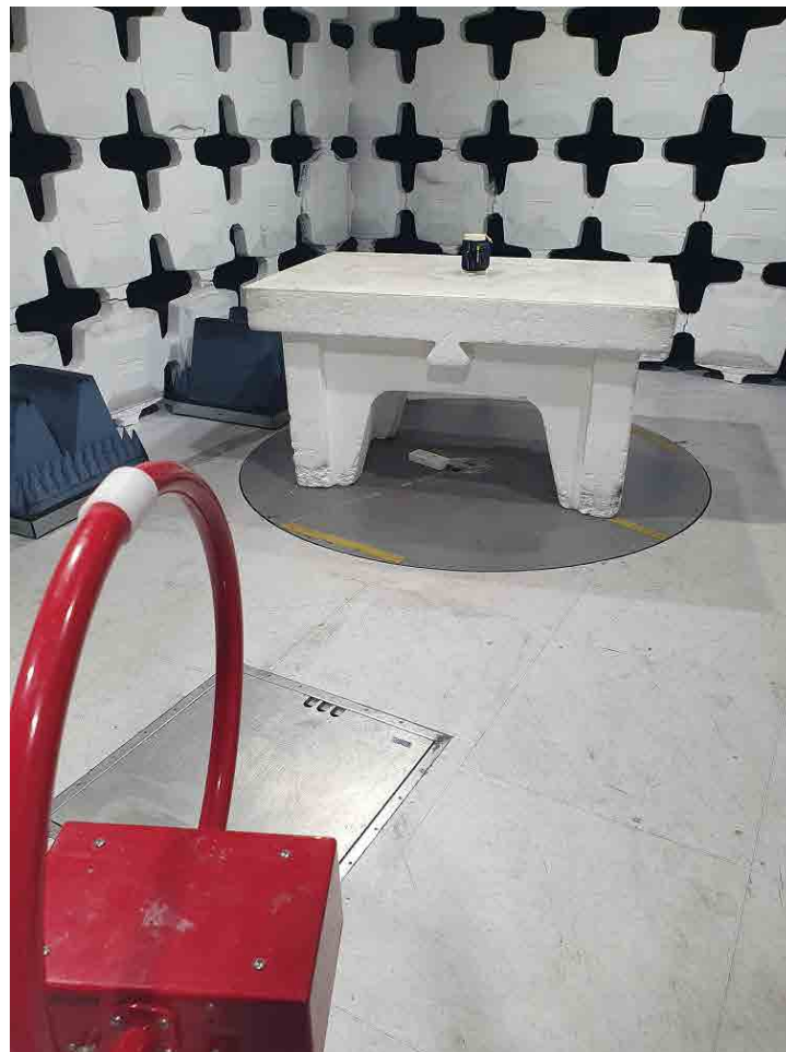
Picture # 6. Radiated Emission test setup below 30 MHz.
