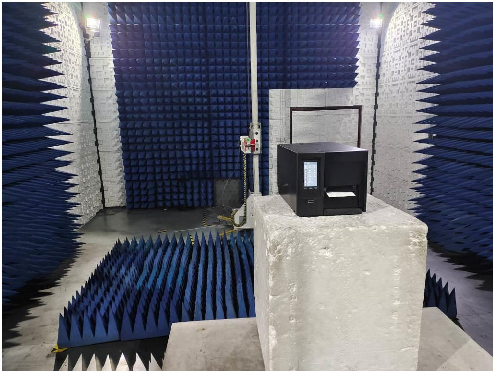
RADIATED EMISSION TEST SETUP ABOVE 1GHz
