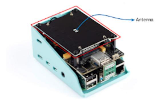
This antenna has been specifically designed and produced by Sixfab engineers, focusing on 5G bands and frequencies, exclusively for the Jumpstart 5G product.
