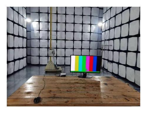
RADIATED EMISSION ABOVE 1G TEST SETUP
