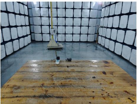
RADIATED EMISSION ABOVE 1G TEST SETUP
