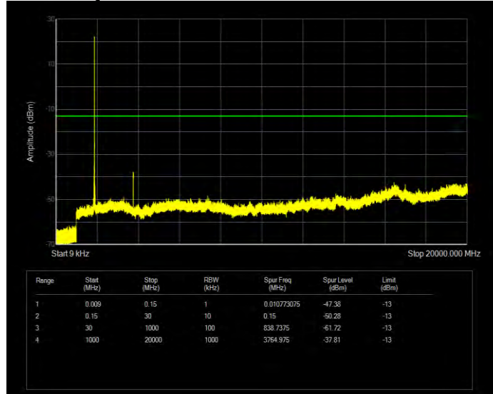
Band25 16QAM BW=3MHz Channel=26675 RB Size=15 Position=#0
