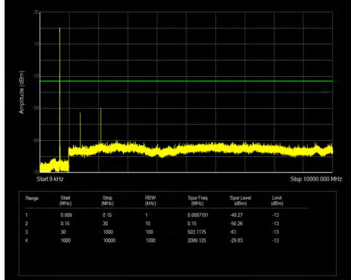
Band12 QPSK BW=1.4MHz Channel=23095 RB Size=6 Position=#0
