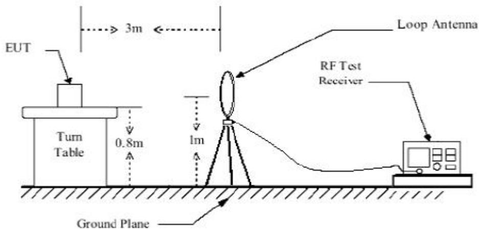
For radiated test from 30MHz to 1GHz
