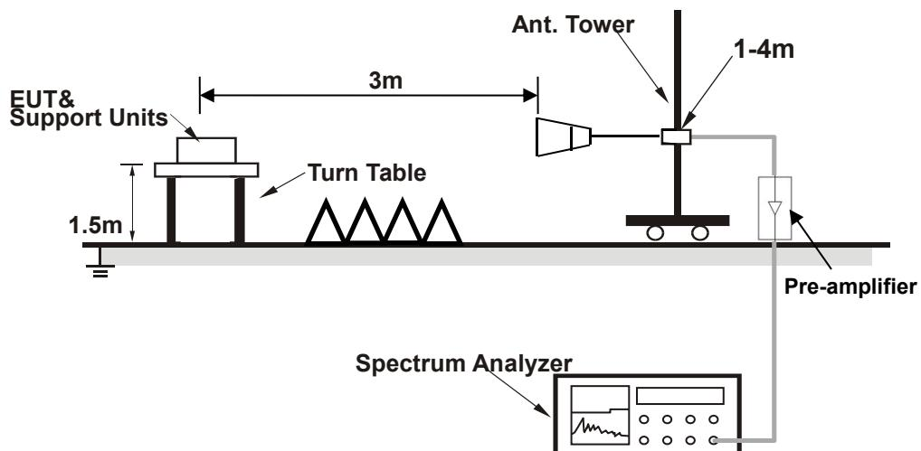
**For radiated test above 18GHz**
