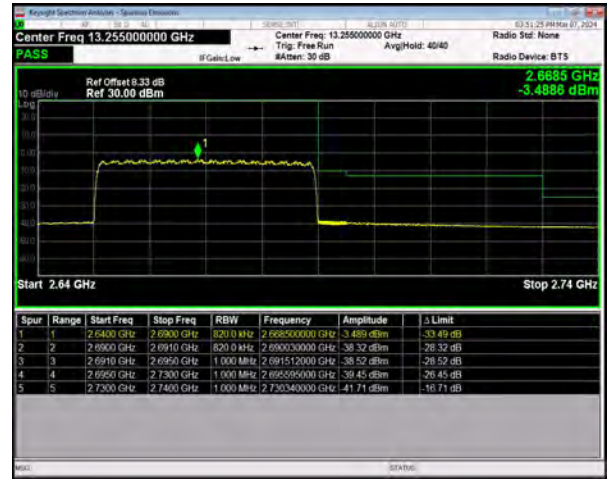
n1 SCS=30kHz CP_QPSK BW=40MHz HighChannel=534000 RB=106@0
