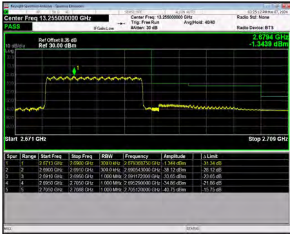
n41 SCS=30kHz DFT_QPSK BW=15MHz HighChannel=536496 RB=36@0
