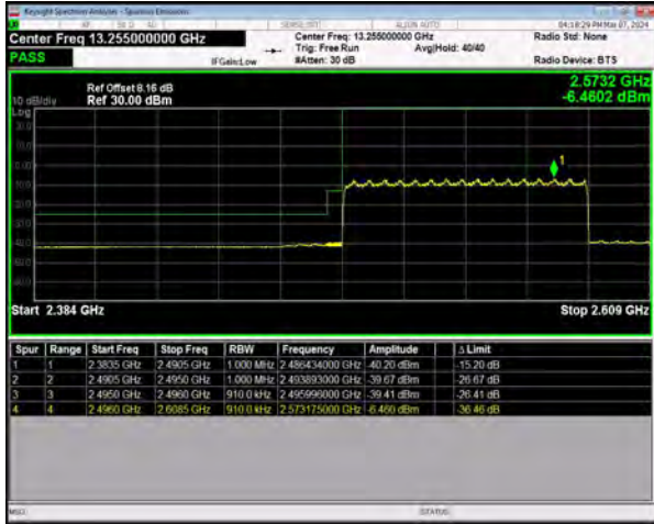
n41 SCS=30kHz CP_QPSK BW=90MHz LowChannel=508200 RB=245@0
