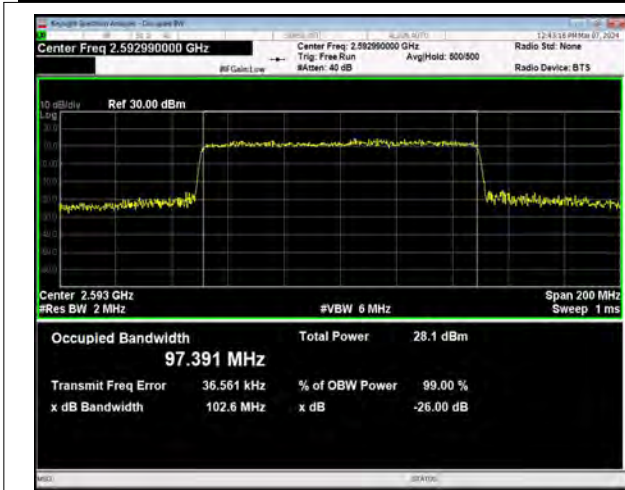
n41 SCS=30kHz CP_64QAM BW=100MHz Channel=518598 RB=273@0
