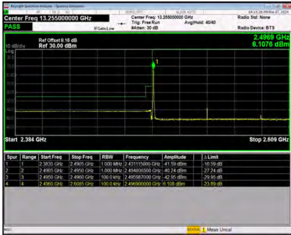
n41 SCS=30kHz DFT_16QAM BW=90MHz LowChannel=508200 RB=1@0
