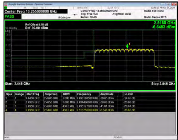
n41 SCS=30kHz DFT_16QAM BW=40MHz LowChannel=503202 RB=100@0
