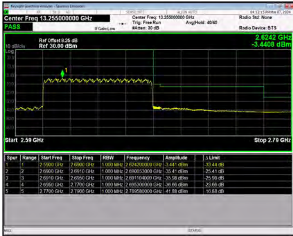
n41 SCS=30kHz DFT_QPSK BW=80MHz HighChannel=529998 RB=216@0
