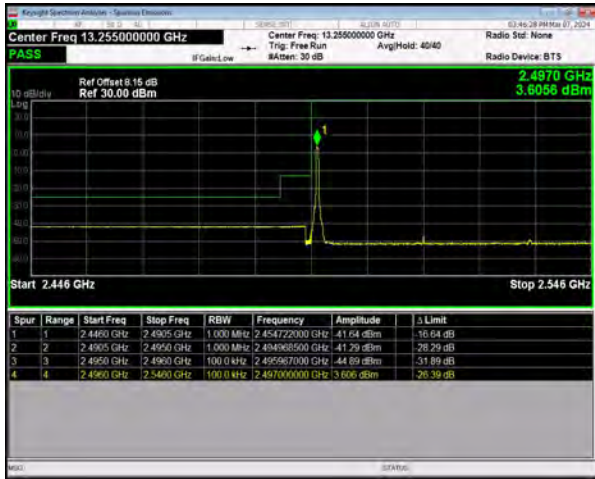
n41 SCS=30kHz DFT_256QAM BW=40MHz LowChannel=503202 RB=1@0
