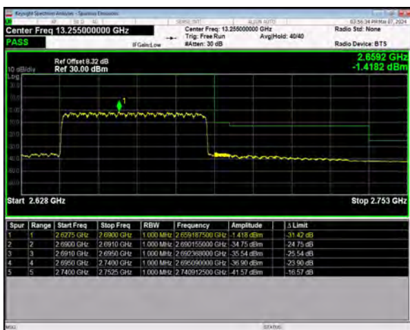
n41 SCS=30kHz DFT_QPSK BW=50MHz HighChannel=532998 RB=128@0
