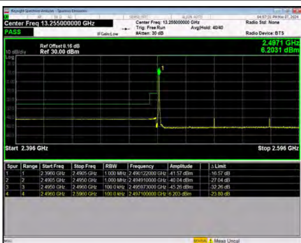
n41 SCS=30kHz DFT_BPSK BW=80MHz LowChannel=507204 RB=1@0
