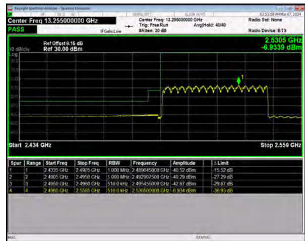
n11 SCS=30kHz DFT_64QAM BW=50MHz LowChannel=504204 RB=128@0
