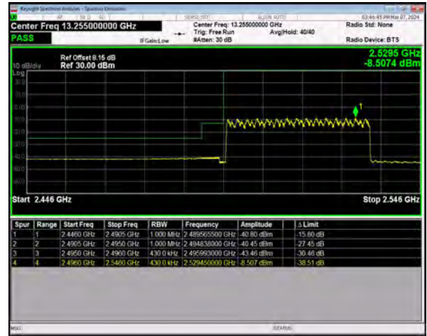
n41 SCS=30kHz DFT_256QAM BW=40MHz LowChannel=503202 RB=100@0
