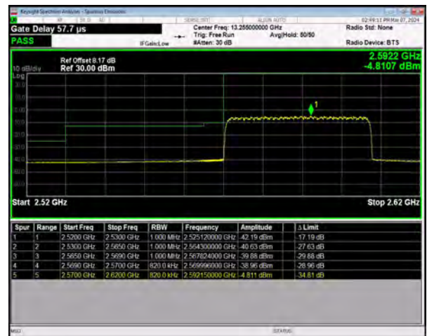
n38 SCS=30kHz DFT_256QAM BW=40MHz LowChannel=518000 RB=100@0
