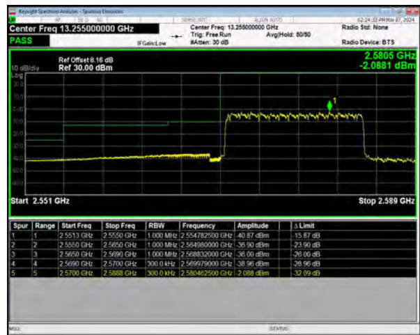
n38 SCS=30kHz DFT_16QAM BW=15MHz LowChannel=515500 RB=36@0
