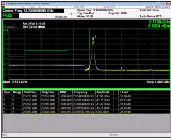
n38 SCS=30kHz DFT_256QAM BW=15MHz LowChannel=515500 RB=1@0
