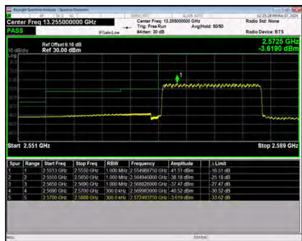
n38 SCS=30kHz DFT_64QAM BW=15MHz LowChannel=515500 RB=36@0
