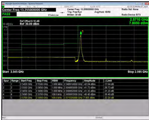
n38 SCS=30kHz DFT_64QAM BW=20MHz LowChannel=516000 RB=1@0
