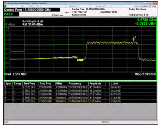
n8 SCS=30kHz DFT_64QAM BW=10MHz LowChannel=515000 RB=24@0
