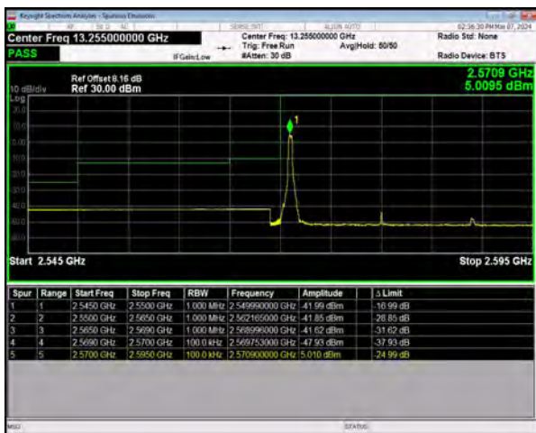
n38 SCS=30kHz DFT_256QAM BW=20MHz LowChannel=516000 RB=1@0
