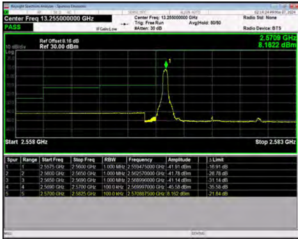
n8 SCS=30kHz DFT_64QAM BW=10MHz LowChannel=515000 RB=1@0
